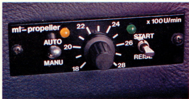
The prototype's electric propeller control allows fingertip adjustment of engine rpm or the option of manual pitch adjustment.
